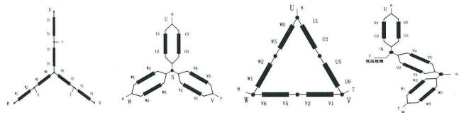
Output voltage (L-L) output voltage (L-L) output voltage (L-N) 400V/50Hz 200V/50Hz 230V/50Hz 220V/50Hz 450V/60Hz 225V/60Hz 260V/60Hz 220V/50Hz
