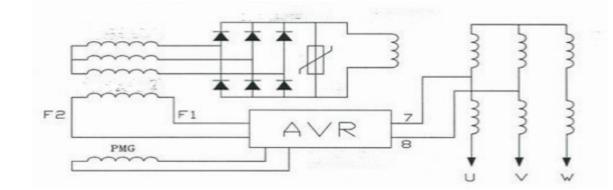
2.2 permanent magnet generator (PMG) excitation-AVR control generator
